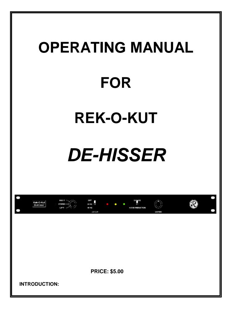
The *Rek-O-Kut De-Hisser* is designed to remove annoying hiss and noise from both old and new phonograph records as well as tape recordings of many formats. It incorporates an input switch which can select either the left or right wall of a mono groove, and also a low-cut, or rumble filter.
